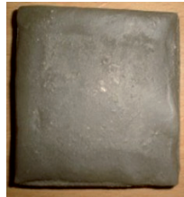
Figure 1. Functionally graded core sample drawn out of mold
