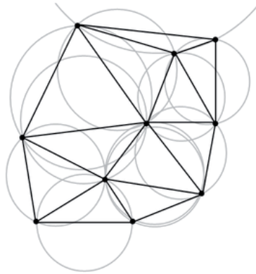
Figure 1. A Delaunay triangulation in the plane with circumcircles.
