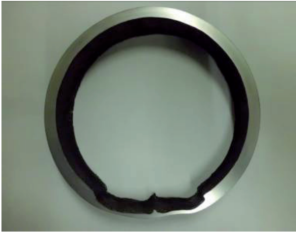
Figure 10. Results of macroetching showing the absence of ERW.
